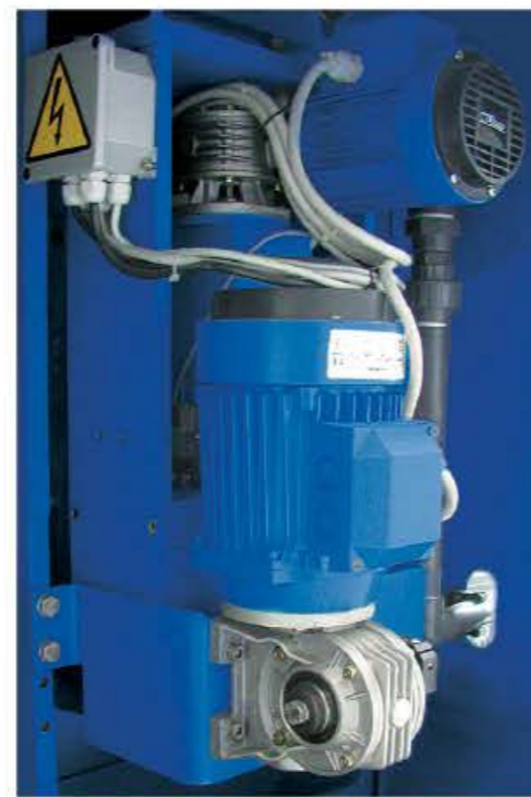
High frequency lateral oscillation system.
